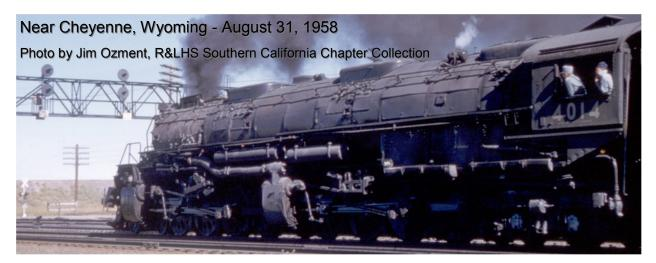
Number 4014 is one of 25 Big Boy locomotives built exclusively for Union Pacific Railroad. Numbers 4000 through 4019 were built in 1941. Five additional locomotives numbered 4020 through 4024 were built in 1944. With a 4-8-8-4 wheel arrangement, they were the largest steam locomotives ever built.
