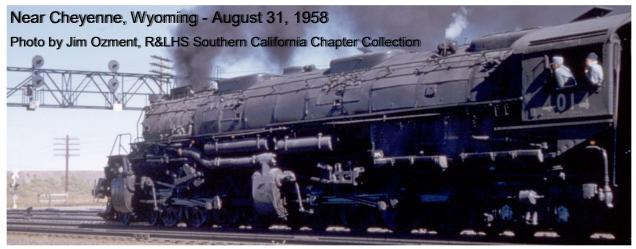
Number 4014 is one of 25 Big Boy locomotives built exclusively for Union Pacific Railroad. Numbers 4000 through 4019 were built in 1941. Five additional locomotives numbered 4020 through 4024 were built in 1944. With a 4-8-8-4 wheel arrangement, they were the largest steam locomotives ever built.
