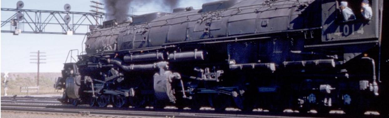
Number 4014 is one of 25 Big Boy locomotives built exclusively for Union Pacific Railroad. Numbers 4000 through 4019 were built in 1941. Five additional locomotives numbered 4020 through 4024 were built in 1944. With a 4-8-8-4 wheel arrangement, they were the largest steam locomotives ever built.
